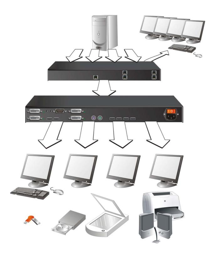
DVI-D CATx KVM-Extender – with full USB 2.0 high speed access
