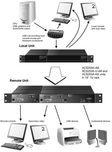
Figure 23 Dual Head application with PS/2, USB and audio/serial extension
