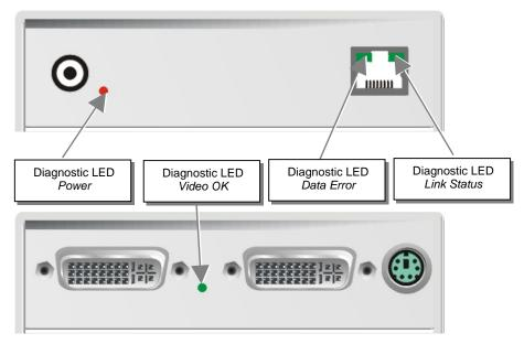
Diagnostic - LEDs at DVI-D Cat X - Extender
