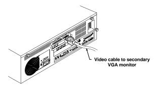
Figure 3-5. Attaching a secondary monitor to the ServLINK for a direct video feed.
