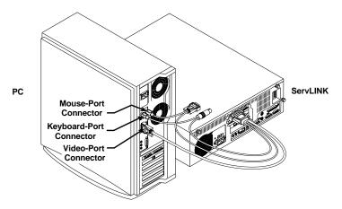
Figure 3-3. Attaching the CPU-extension cable to a CPU (a PS/2 type CPU is shown).
