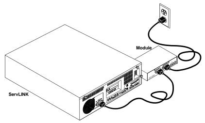
Figure 3-10. Attaching the power cords.
