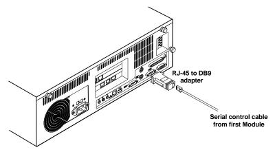
Figure 3-11. Attaching the cable from the first PC's Module to the ServLINK.
