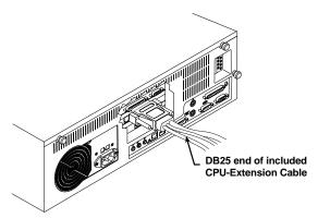
Figure 3-2. Attaching the CPU-extension cable to the ServLINK.
