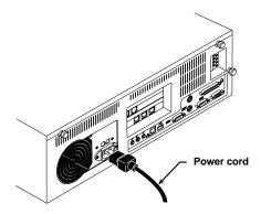
Figure 3-14. Attaching the power cord to the ServLINK.
