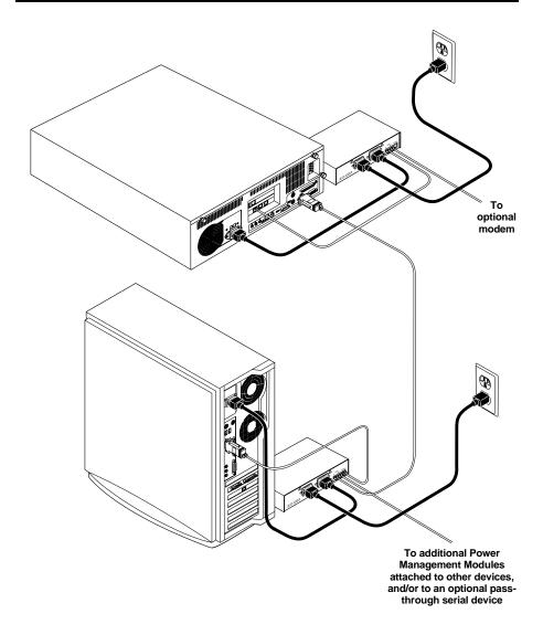
Figure 3-13. A ServLINK system with Management Modules installed.
