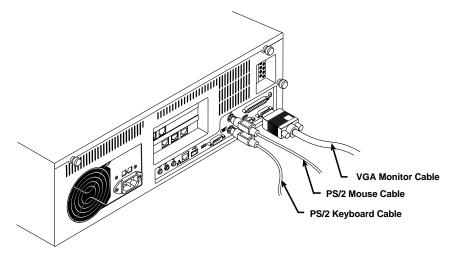
Figure 3-1. Attaching the peripherals to the ServLINK.
