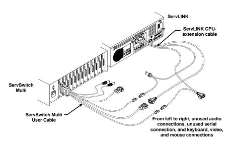
Figure 3-4. Attaching the CPU-extension cable to a KVM switch with composite user ports (the ServSwitch Multi is shown).
