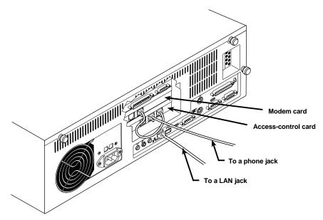
Figure 3-6. Attaching the ServLINK to the public phone network or a LAN.
