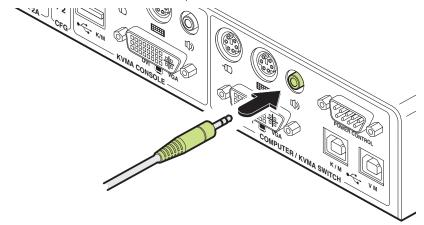
2 Connect the plug at the other end of the audio link cable to the speaker / line out socket of the host computer or KVMA switch.
