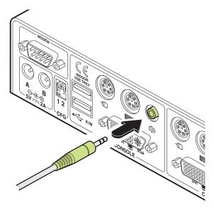
2 Connect the main speaker cable to the port labelled (\*) within the KVMA CONSOLE section of the rear panel.
