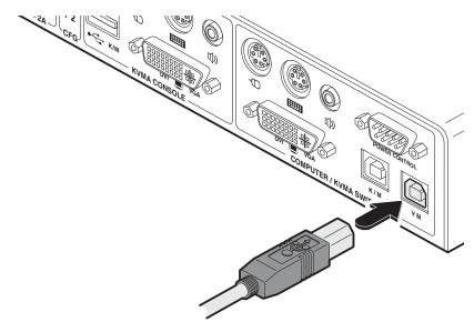
2 Connect the plug at the other end of the USB link cable to a vacant USB socket on the host computer or KVMA switch.
