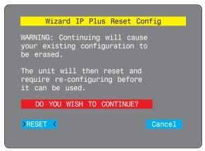
5 Remove power, return the mini switch 1 to its OFF position and then reapply power. The locally connected monitor should display the first screen of the <u>initial configuration sequence</u>.
