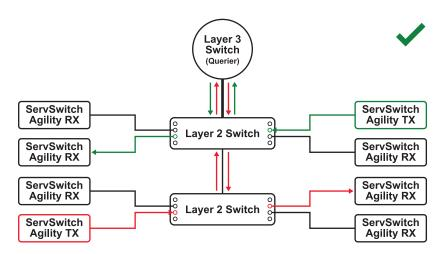
Figure 2-3. Line cascade layout with data paths.
