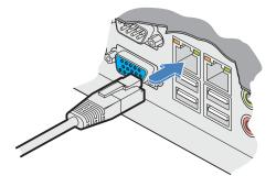
Figure 3-1. Connecting Category 5, 5e or 6 cable from LAN / network switch.
