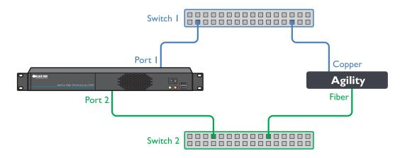
The 'Separate Device Networks' option mentioned earlier would be enabled on the iPATH Agility Controller and the respective network connections on the endpoints are connected accordingly (e.g. copper to copper on only switch 1 and SFP to SFP only on switch 2).
