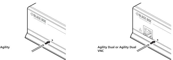
After roughly eight seconds, when the factory reset has completed, five of the front panel indicators will flash for a period of three seconds to indicate a successful reset operation.
