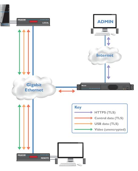
Figure 2-2. Transport Layer Security data diagram
