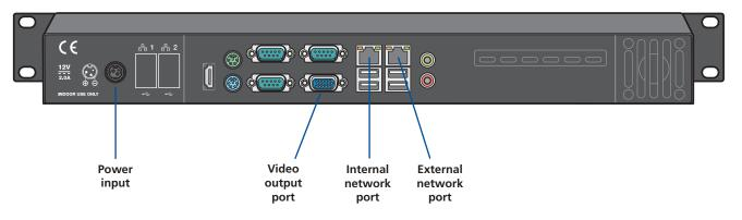
Figure 2-5. iPATH Agility Controller unit - rear panel. During normal use, only the network and power connections are used.
