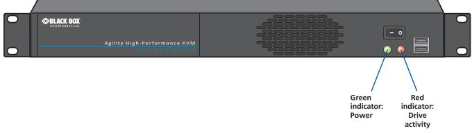
Figure 2-4. iPATH Agility Controller unit - front panel.
