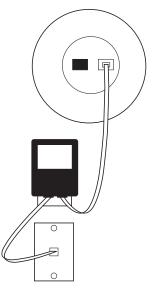
When the Voice Conferencing System is plugged in correctly, the two LEDs on the main module will be solid red. This indicates that the Voice Conferencing System is receiving power. If the LEDs do not light, make sure that the power-interface module is securely plugged into a working outlet—check the outlet by plugging a lamp into it if necessary—and that the modular cable with the RJ-45 connectors is securely plugged into both the main module and the power-interface module.
