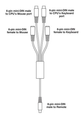
Figure 5-12. The Remote Local Workstation Keyboard/Mouse In/Out cable.
