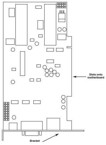
Figure 3-1. The Supervisor PCI Card.
