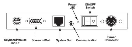
Figure 5-2. Ports on the Supervisor Box.
