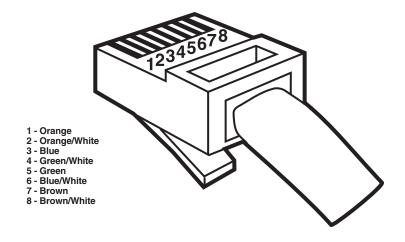
Figure 5-4 illustrates the RJ-45 male pinout and wire diagram.
