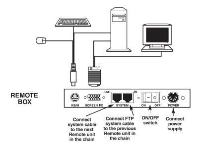
Figure 5-19. The ClassWork Junior Remote Box system connections.
