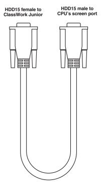
Figure 5-10. The Remote Unit Local Workstation Screen cable.
