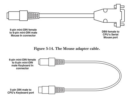
Figure 5-15. The Keyboard In adapter cable.
