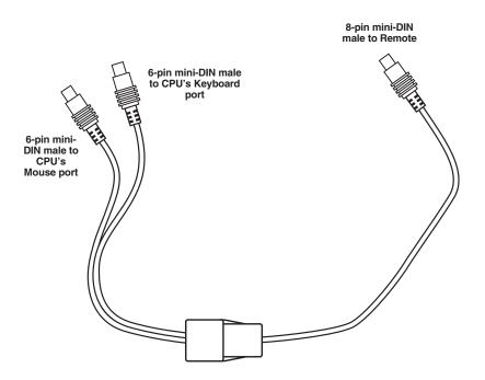
Figure 5-9. The Remote Local Workstation Keyboard/Mouse In/Out Cable.
