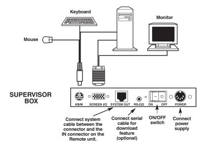
Figure 5-18. The ClassWork Junior Supervisor Box system connections.
