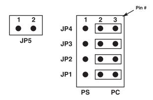
Figure 4-1. Jumper Settings for AT Mouse.
