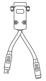
Fig. 3-14. Keyboard Cable for PS/2.
