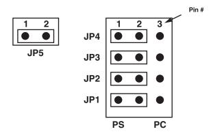
Figure 4-2. Jumper Settings for PS/2 Mouse.
