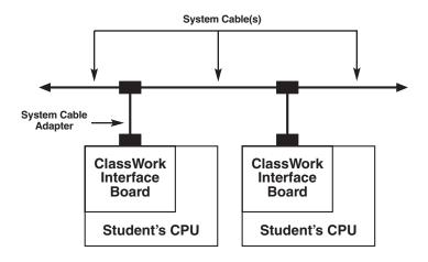
Figure 4-8. System Cable Adapter Connections.
