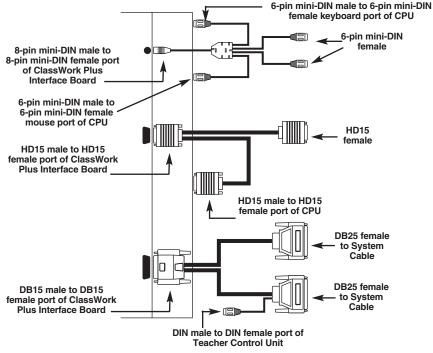
Figure 4-21. Cable Diagram for PS/2 Connections.
