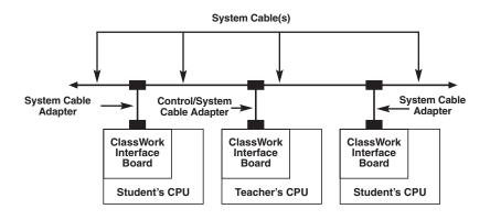
Figure 4-19. System Cable Connections.
