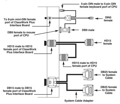
Figure 4-9. Cable Diagram for AT Mouse Connections.
