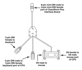
Figure 4-13. I/O Adapter for AT Mouse.
