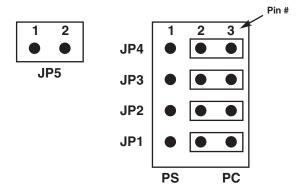
Figure 4-11. Jumper Settings for AT Mouse.
