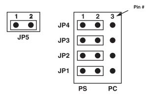
Figure 4-12. Jumper Settings for PS/2 Mouse.
