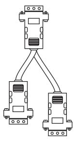
Fig. 3-10. Serial Mouse Cable.
