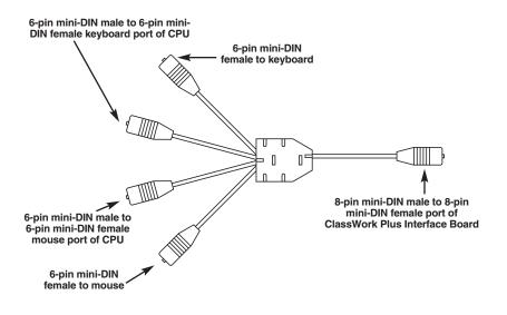
Figure 4-14. I/O Adapter for PS/2.
