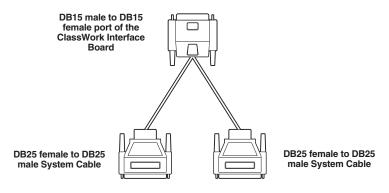
Figure 4-6. System Cable Adapter.
