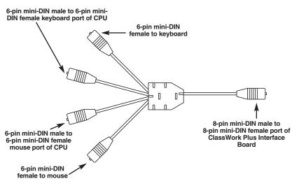
Figure 4-4. I/O Adapter for PS/2.
