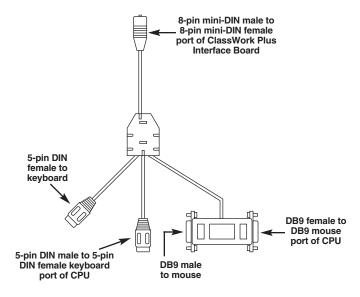
Figure 4-3. I/O Adapter for AT Mouse.
