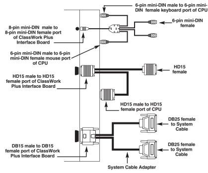
Figure 4-10. Cable Diagram for PS/2 Connections.
