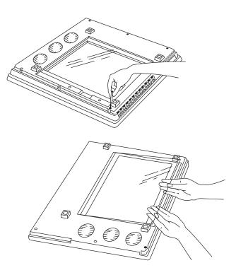
Removing the Bottom Glass for Cleaning.
