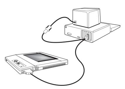
Fig. 2. Connecting the Y Cable.
