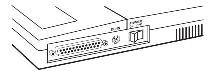
Fig. 1. Connectors and Switch on the LCD Panel.
