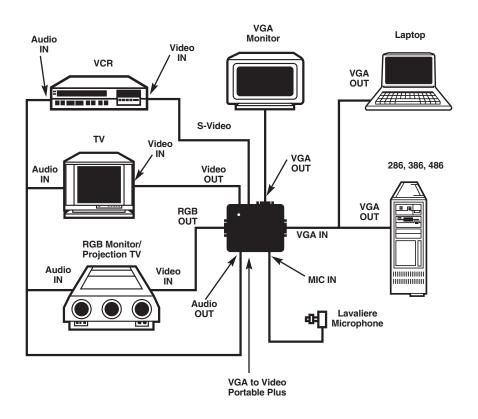
Figure 2. VGA to Video Portable Plus System Connections.
