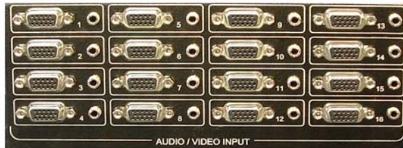
Figure 2 - Audio and video inputs on AC1123A
