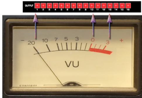
Figure 11 –Comparison with Analog VU meter on 16x16 Matrix
