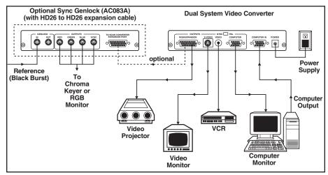
Figure 1. The Dual System Video Converter allows you to output your computer monitor signal to three video devices.
