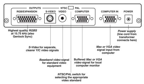
Figure 2. Rear panel of the Dual System Video Converter.
