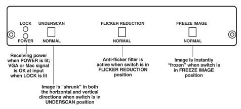
Figure 3. The front panel of the Dual System Video Converter.
