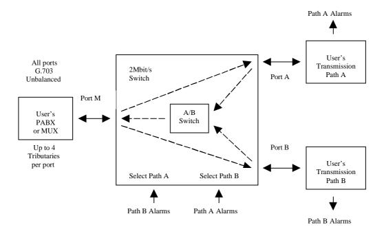
The switch is powered from either a 24 or 48 Volt nominal DC supply of either polarity. Each port has four inputs and four outputs. Each traffic interface is G.703 unbalanced 75 ,Type 43 connectors. The inputs at port M feed the A and B ports via a buffer. The output at Port M is either from Port A or Port B depending on the position of the internal A/B switch - which in turn is driven by the external inputs (i.e. the occurrence of an alarm event - AIS/LOS etc).
