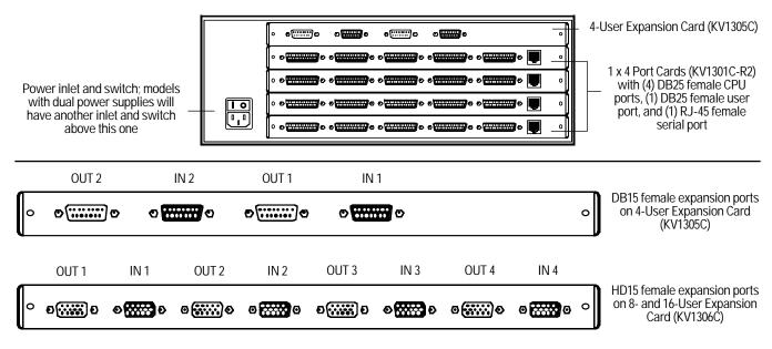
On the 4-user expansion cards (above, top), IN 1 and OUT 1 carry signals for the port cards in slots 1 and 2, while IN 2 and OUT 2 carry signals for the port cards in slots 3 and 4.
