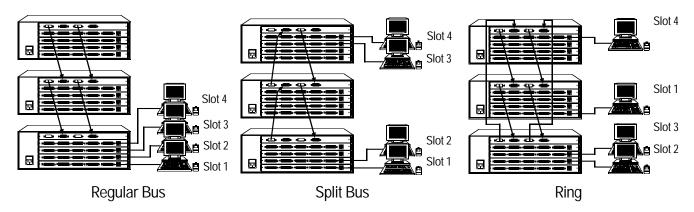
\*Keep in mind that only one user at a time can use the bus that interconnects daisychained Affinity units, especially when you implement a ring topology. For example, when your Affinity units are interconnected in a ring, if any user on slot 1 selects a CPU attached to an Affinity unit other than his own, no other slot 1 user can select any CPUs.
