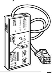
The Token Ring Test Kit detects either shielded twisted-pair (STP) or unshielded twisted-pair (UTP) cabling assembly errors.
